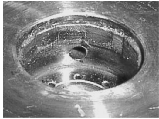
Fig. 5 Discharge chamber after the 1200-h preliminary endurance test. No significant sputtering damage or deposition of sputtered material inside the discharge chamber. (The hole under the Sm-Co magnets on the inner wall is for installing a plasma ignitor.)
